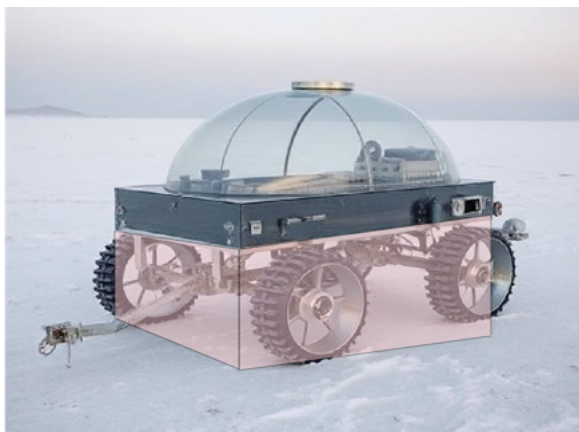
Figure 5: An artistic conception that visualizes the essential elements. A Fresnel-lens dome would be close to the ground to focus the light and act to trap the newly released water vapor. Water vapor in the canopy would find a cold trap and deposit. Later, the cold trap could be skimmed or even warmed to collect the H_2O molecules into a better container for transport or long-term storage.
